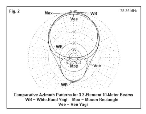
The patterns reveal something else about what happens when you Vee and element horizontally. The front-to-side ratio goes way down, since each half element radiates some energy to the side.
