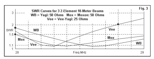
The wide-band Yagi 50-Ohm SWR curve may start higher than the other two, but only because the antenna provides coverage of the entire 10-meter band from 28.0 to 29.7 MHz. You can lengthen the driver slightly to bring the minimum SWR value down in frequency.
